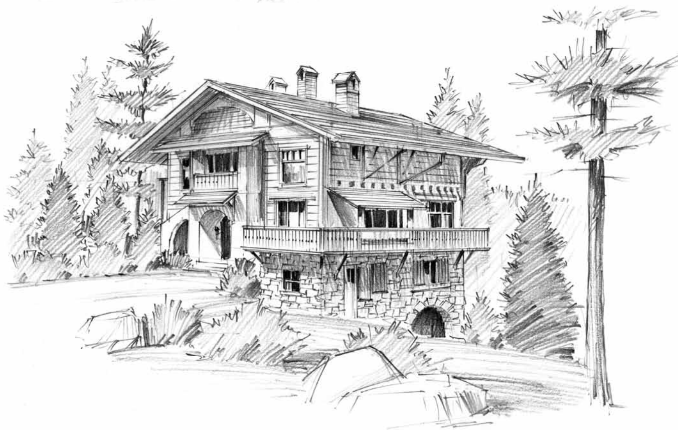
SIMPLE ROOF FORMS SHELTERING FULL BUILDING
