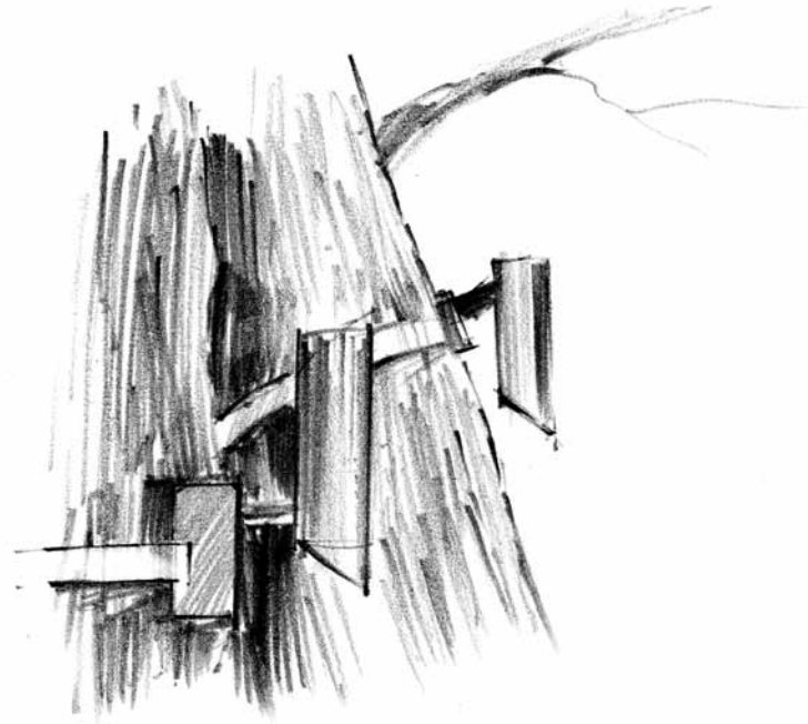
DIRECTIONAL DOWN LIGHTING FROM MATURE TREES CAN BE ACHIEVED THROUGH SPECIAL MOUNTING HARDWARE
